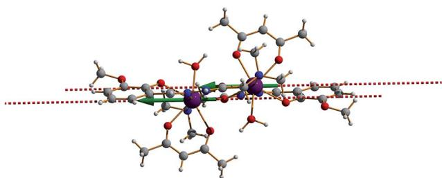
Fig. 5 Orientations of the anisotropy axes (dashed line) in **2**. Colour scheme: Dy-purple, O-red, C-grey, N-blue, H-white. Green arrows represent the orientation of the local magnetic moments on Dy<sup>III</sup> sites in the coupled ground state, arrangement driven by ferromagnetic dipolar coupling.
