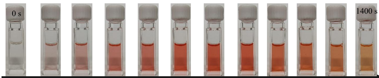
Figure S42. Color change of the solution of 2,2'-mPCL in 1,4-dioxane during UV irradiation at different points in time: 0, 5, 10, 20, 30, 60, 90, 120, 180, 300, 560, and 1400 s.
