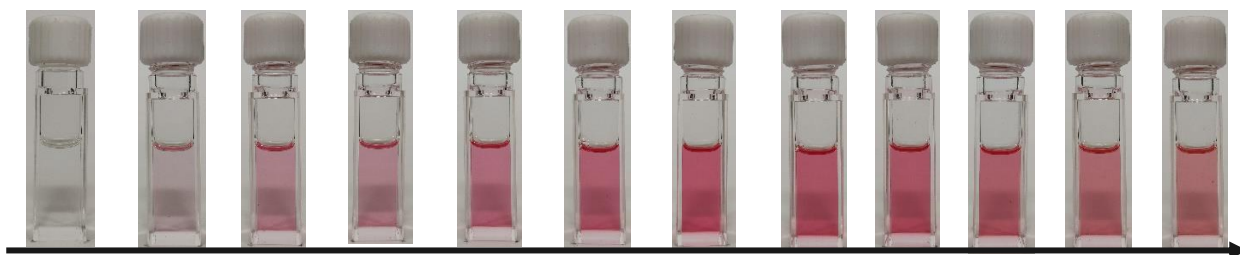
Figure S44. Color change of the solution of 5,5'-mPCL in 1,4-dioxane during UV irradiation at different points in time: 0, 5, 10, 20, 30, 60, 90, 120, 180, 300, 560, and 1400 s.
