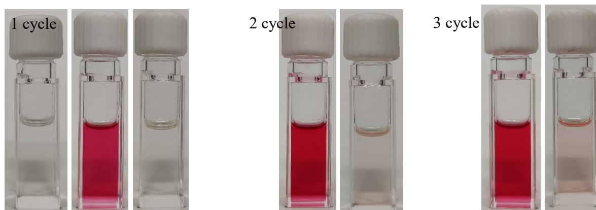
Figure S48. Color change of the solution 5,5'-mPCL in 1,4-dioxane during 3 cycles of UV irradiation for 1.5 min and ultrasonication.
