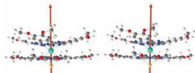
Fig. S300. [4]^{4+} Tb2 (a): plot of the fragment of the quadruple-decker (overall oxidation state +4) used in the ab initio calculation, together with the calculated easy axis direction. Crystallographically distinct Tb(III) ion Nr. 2 (SP coordination). Nr. of electron pairs in calculation: 444.
